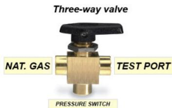
Likewise, a 3-way valve could be positioned to perform the same function. This would put the gas pressure immediately below the switch to atmospheric pressure. The unit should not be able to light off. In this case, an external pressure source could then be connected to the vent port, and with the palm valve being held open, the switch could be pumped up to its set point in an accurate manner until a volt ohm or continuity tester indicated a switch trip.
