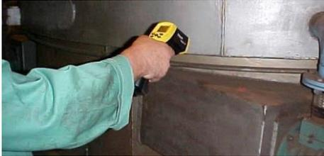
Whenever an electrical circuit carries a load, the current passing through the circuit creates heat. This heat is a function of the resistance encountered. Any increase in flow or resistance will generate more heat.
