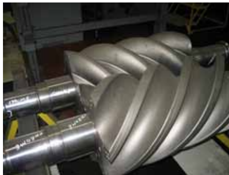
Figure 8-1 Rotary Screws Used in Air Compressor System
