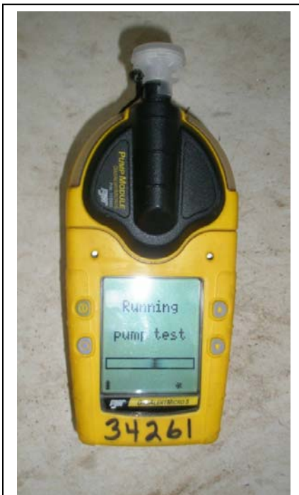
Picture 03: LEL Meter
