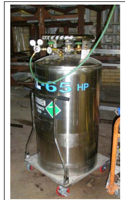
Picture 02: Nitrogen Tank
